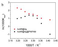
Fig.1 (a) TEM image, (b) catalytic activity with different temperature
